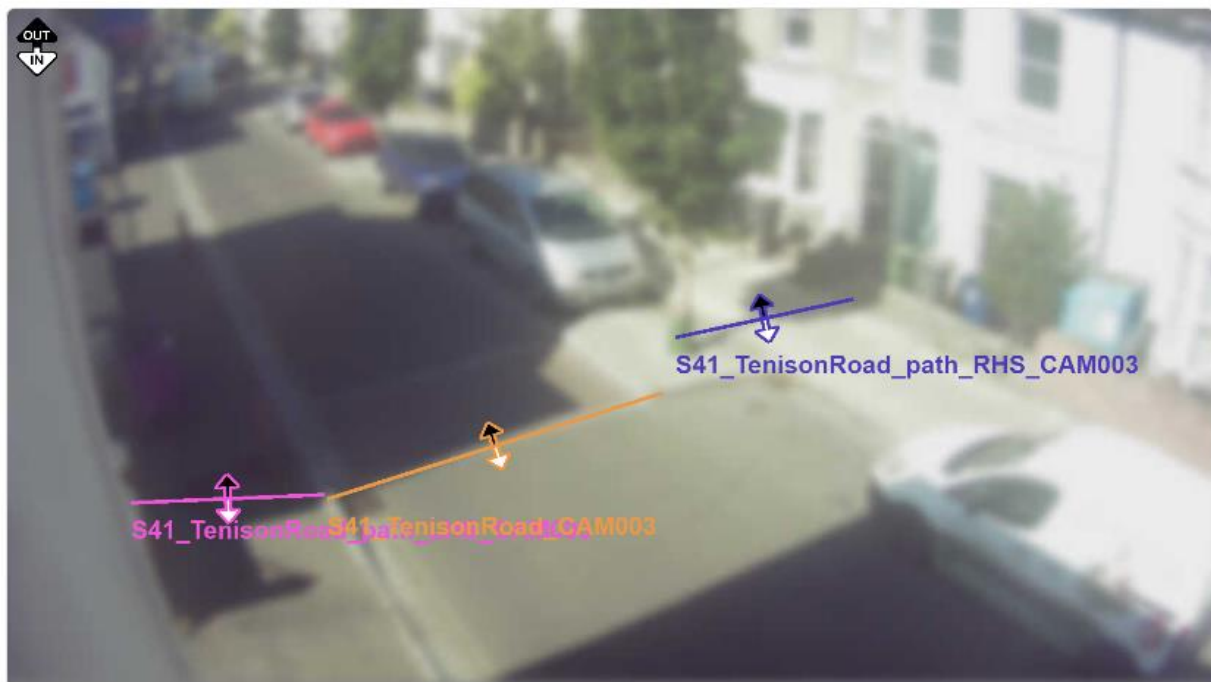
Figure 2: The Tenison Road sensor field of view. The sensor has three countlines: a main road countline and two pavement countlines (Tenison Road S41, Lens 1 view, Vivacity dashboard, 08.07.2022).
